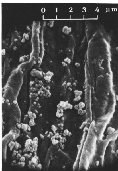
Figure 15. Scanning electron micrograph; paper fiber bearing modern pine soot ink having a bluish tone
