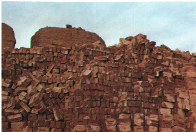
Figure 8. Color variations in contemporary brick formed of Tigris River deposited clay and fired in a scove kiln near Baghdad
