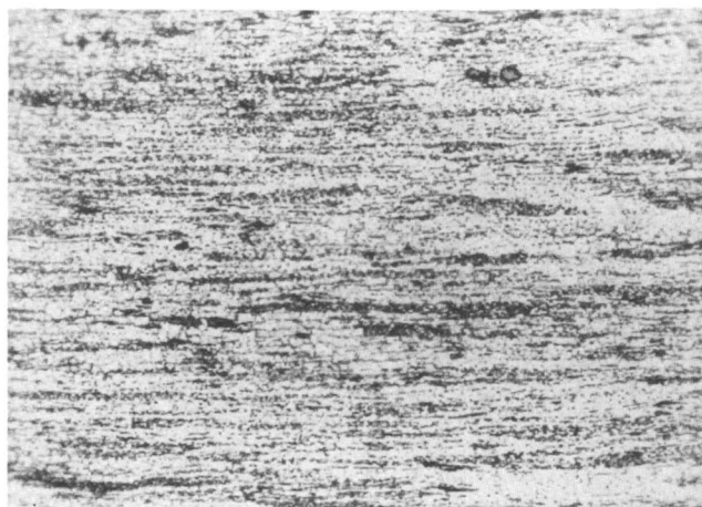
Figure 4b. Transverse section from edge of a fracture in the back of the head of the Female Head (private collection). Structure illustrates the "banded" structure produced by a considerable amount of deformation by hammering ( \times 225 ).
